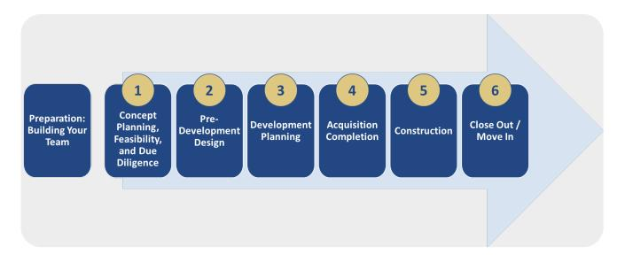
The six phases of the real estate development process build on each other, starting with a development concept and ending with a finished structure. While these phases are presented in an orderly flow, activities often begin in one phase and end in another.
